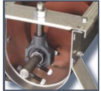
Auger suspended in adjustable ball bearings
